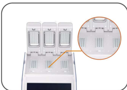
Long service life Peltier heating units
