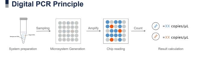
The strategy of digital PCR - "divide and rule". A standard PCR reaction is allocated to a large number of micro reactors, and each reactor contains or does not contain one or more copies of the target molecule (DNA template) to achieve "single molecule template PCR amplification". After amplification, the number of positive wells is "counted" by the number of positive reactors, and then the number of positive copies is calculated according to Poisson's formula.
