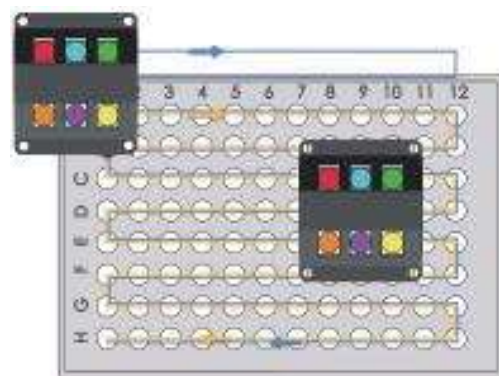
Innovative time-resolved well-by-well scanning pattern
