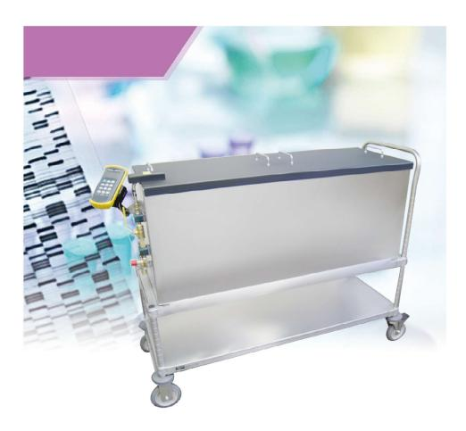
The inner wall of UM50 series sample fumigation operating vehicle adopts corrugated cooling structure to ensure the balance of ambient temperature; High vacuum thermal insulation, multi-layer thermal insulation, reduce evaporation of liquid nitrogen; With flat structure and open design, the samples taken from the liquid nitrogen tank can be conveniently boxed, numbered and scanned.
