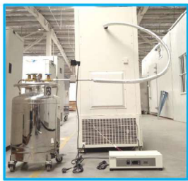
LN 2 /CO 2 backup system
