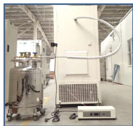
LN 2 /CO 2 backup system
