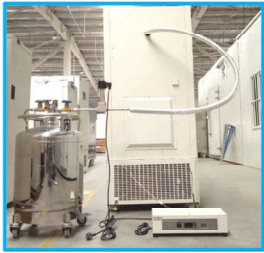
LN 2 /CO 2 backup system
